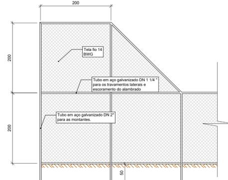
DETALHE TÍPICO DO ALAMBRADO NA LATERAL
